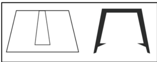
Figure 3. Frustum Preparation and The Internal Metal Protrusion.
