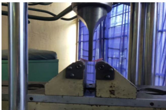
Figure 1. Transverse strength testing of heat cured acrylic resin plates
