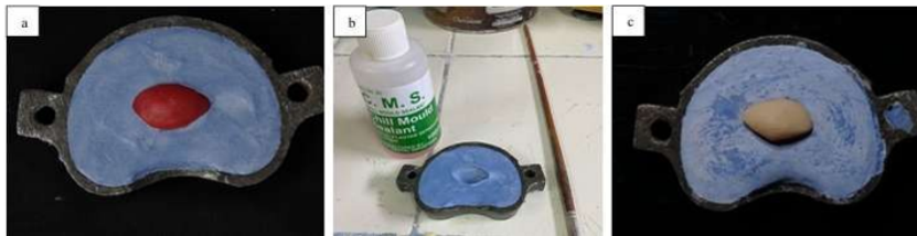
Figure 2. Laboratory procedure: A. Investing, B. Application of separating agent, and C. Deflasking the acrylic sclera.
